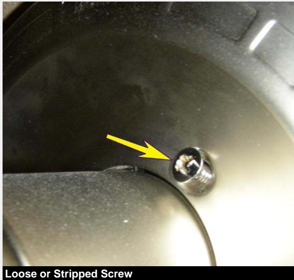
Loose or Stripped Screw
